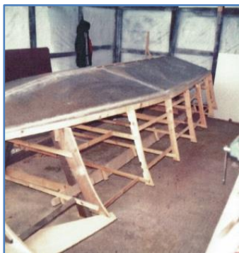
The hull plug at an early stage.
